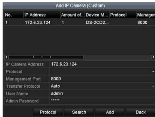
Figure 2-39 Custom Adding IP Camera Interface
