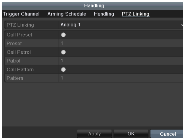
Figure 8-7 Set PTZ Linking of Alarm Input
